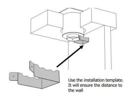
2. Install the ceiling cover plate around the Load Bearing Support.
