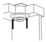
The Ceiling Cover Plate will give the chimney a nice finished look. It covers the gap between the round support and the ceiling.  $\sim$ 7.5» around support box. If the ceiling is at a 90° angle with the chimney, or has a pitch of less than 5°, use the **one piece cover plate**. If it has a greater pitch, chose one of the **2-piece cover plate** versions (see below).
